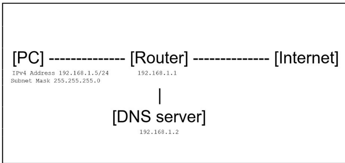
Diagram showing a PC, Router, and the Internet all connected in one row with a DNS server below connected to the router. The PC's IPv4 Address is 192.168.1.5/24 and the Subnet Mask is 255.255.255.0. The Router's IP is 192.168.1.1 and the DNS server's 192.168.1.2
